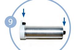
For the column installation, remove dust caps of new column. Make sure there is no dust or debris where the dust caps were located.
