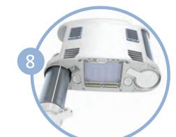
Remove the column completely from the Inogen One® G3. And then repeat steps 5 - 7 for the other column.
